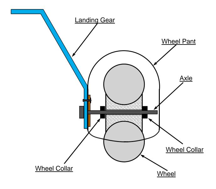
STEP 1: Install wheel pants with typical installation
