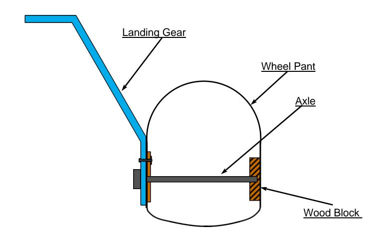
STEP 3: Glue the wood block the wheel pants using epoxy, making sure the wheel pants screws are tight, the wheel pants are seated in their "natural" position, with no stress on the fiberglass. If using a soft wood, it is helpful to harden the wood at the hole for the axle with thin CA.
