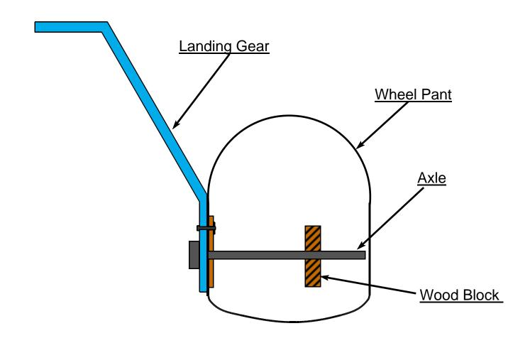
STEP 2: Make a small block of wood (balsa or lite ply) about 1"x1-1/2"x1/4", and drill a hole the size of the axle in the center.
