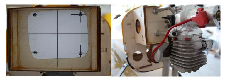
We recommend 4/40 push rods for throttle and/or optional choke servo. Also ensure there is no metal-tometal contact from the throttle/choke to the servos. 2/56 Ball links for 4/40 rod (not included) will prevent the aforementioned metal-to-metal contact and will bolt to nicely to your motors carburetor.
