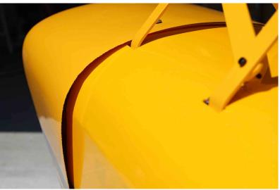
□ Once satisfied the paint lines are matched to the fuse and you have the same amount of gap on each side, drill and install your remaining 4/40 cowl bolts.
