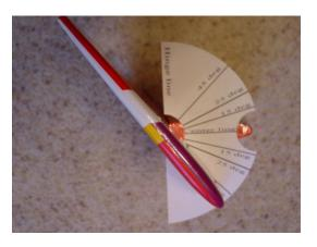
CG Range is 7-1/2 to 7-3/4 inches back center of the top wing or dead center of the rear cabane.
