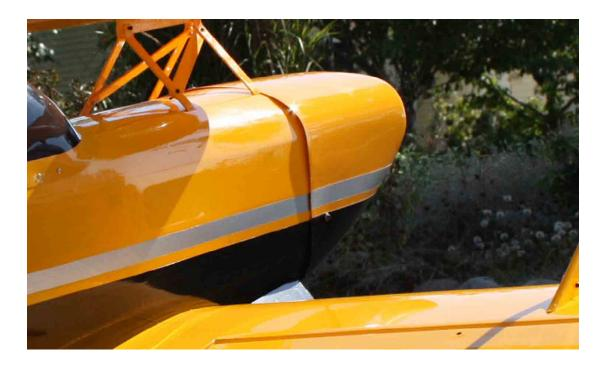
Note the gap between the cowl and fuse. Remember to keep it even on both sides to achieve the proper look.
