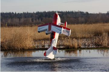
Every airplane has structural limits, and the larger the plane is, the more critical it is to understand and respect these limits. This is particularly true for 3D aerobatic planes, since by design, these planes are light weight, are over powered, and have oversized control surfaces.
