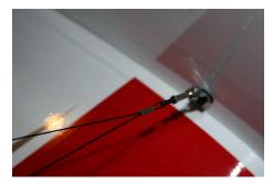
□ Now with each loose wire end, slide on a crimping swag (see first picture below). Now run the wire through the eyelet and back though the crimping swag and push the swag up to the eyelet at the top of the strut (see second picture below). You will have just a little slack in the wire at this time.
