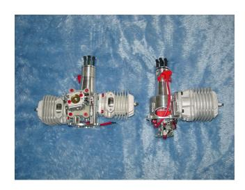
Also with the engine is installed, you will want **7-11/16** inches from the firewall to the spinner back plate for proper cowl placement.
