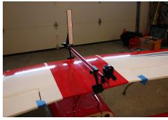
☐ If satisfied with the incidence, remove the top wing and struts and epoxy in the tabs with the struts attached the same way you did the lower wing. Remove the struts before the epoxy has set and clean up any epoxy that may have oozed out.
