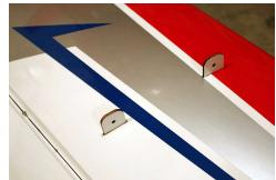
□ Now for the top wing. Before you glue in anything you are going to want to check wing incidence. The incidence for this aircraft is 0 degrees for the motor, 0 for the stabs and lower wing. The upper wing needs to be at negative -1.5 degrees. These aircraft are built on jigs and the incidence is preset but it's still a good idea to check it so there will be no surprises during your maiden.
