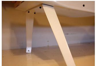
☐ Install the landing gear to the fuselage using the four 8/32 bolts, spring washers, and flat washers, and compression nuts.
