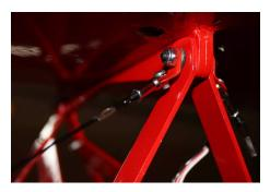
During assembly and disassembly, the flying wires always remain attached to the fuse and cabane. Just tuck the flying wire ends into the lower wing tube socket using a piece of foam to keep the wires from falling out during transport. The bolts and tabs should all still be attached, this will greatly cut down on assembly time at the field.
