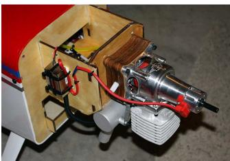
We recommend 4/40 push rods for throttle and/or optional choke servo. Also ensure there is no metal-to-metal contact from the throttle/choke to the servos. 2/56 Ball links for 4/40 rod (not included) will prevent the aforementioned metal-to-metal contact and will bolt to nicely to your motors carburetor.
