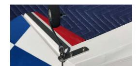
Make sure to align the tail wheel assembly with the sharpest point of the bevel to ensure it doesn't put extra stress on the rudder.
