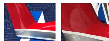
through the horizontal stabilizer slot in the fuselage. Once elevator is in you can now install the horizontal stabilizer using thin CA. Make sure horizontal stabilizer is properly aligned before using any glue.
