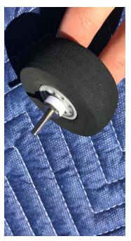
□ Insert wheel axel onto main gear, on the back size use supplied washer and nut. Only thread in the nut until wheel pant in slipped between the axel and main gear. Once wheel pant is properly aligned tighten down nut while holding axel.
