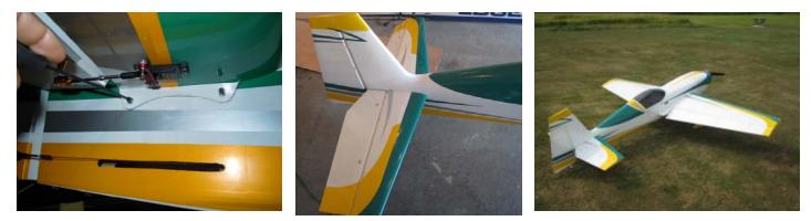
*Tip#8 If the wing is tight you can coat the tube with a little baby powder to aid the insertion of the wing panels.*
