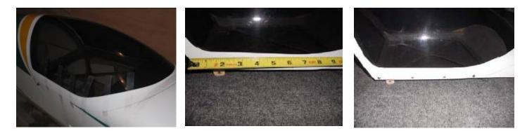
□ Install the canopy using the small wood screws. If satisfied with the fit, remove the canopy and hatch and wick a small amount of thin CA into each of the screws holes on the hatch. Once dried, reinstall canopy with optional canopy glue if desired. The prototype used household Goop Glue to attach the canopy to the hatch, in addition to the small wood screws. **Caution!** CA will fog the canopy if installed before completely drying.
