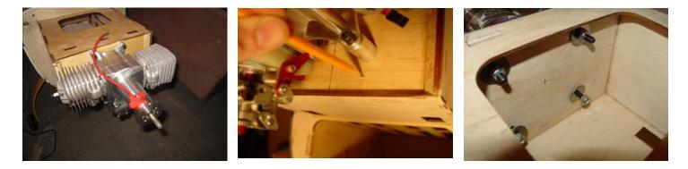
We recommend 4/40 push rods for throttle and/or optional choke servo. Also ensure there is no metal-tometal contact from the throttle/choke to the servos. 2/56 Ball links for 4/40 rod (not included) will prevent the aforementioned metal-to-metal contact and will bolt nicely to your engine's carburetor.
