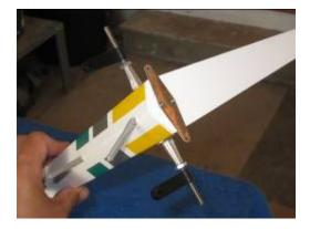
□ Install the tiller springs you set aside in chapter 2 to the tiller horn and tiller.
