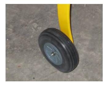
□ Install the landing gear to the fuselage using the four 8/32 bolts, spring washers, and flat washers, and compression nuts.
