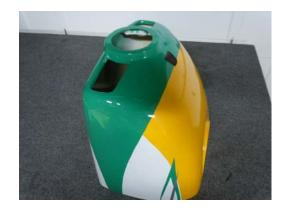
Always wear a mask and eye protection while cutting fiberglass. Take your time while installing the cowl. With care you will end up with a professional installation that will make an impression at the field.
