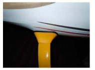
narrow end of the cuffs meets the main gear. Slide the cuffs up until they gently meet the fuse (it is best to leave a 1/16" gap, so the cuffs don't quite touch the fuse, so the cuffs do not damage the belly when the gear flexes). Wipe off possible silicone excess and let cure.
