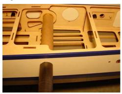
Tip#6: Depending on climate conditions, the wing tube may be too tight or too loose. If the wing is tight you can coat the tube with a little baby powder to aid the insertion of the wing panels. If still too tight, warp a sheet of sand paper around a dowel covered with a foam pad, and sand the inside of the socket. DO NOT sand the CF tube. If too loose, add some wide packing tape to the surface of the wing tube.
