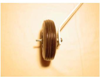
we recommend the use of loc-tite on the setscrews of the wheel collars to prevent them from vibrating loose.
