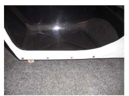
☐ Install the canopy using the small wood screws. If satisfied with the fit, remove the canopy and hatch and wick a small amount of thin CA into each of the screws holes on the hatch. Once dried, reinstall canopy with optional canopy glue if desired. Cauton! CA will fog the canopy if installed before completely drying.
