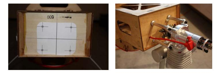
We recommend 4/40 push rods for throttle and/or optional choke servo. Also ensure there is no metal-tometal contact from the throttle/choke to the servos. 2/56 Ball links for 4/40 rod (not included) will prevent the aforementioned metal-to-metal contact and will bolt to nicely to your motors carburetor.
