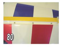
Tip#5 Optional step. After your epoxy has cured, it would be a good time to seal all of your hinge gaps prior to installing the rest of the hardware. This can provide you with a better flying aircraft by increasing control surface performance and preventing possible flutter. Clear or matching covering material can be ironed in place to fill any gaps on the bottom of your control surfaces.
