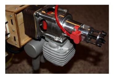
We recommend 4/40 push rods for throttle and/or optional choke servo. Also ensure there is no metal-to-metal contact from the throttle/choke to the servos. 2/56 Ball links for 4/40 rod (not included) will prevent the aforementioned metal-to-metal contact and will bolt to nicely to your motors carburetor.
