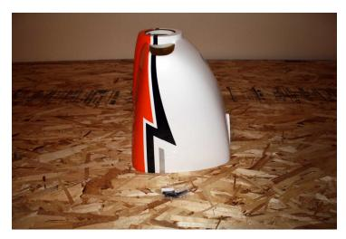
Close the choke and place a piece of tape over the carburetor inlet and exhaust outlet to keep out any dust while setting up your cowl. Since the cowl is preset and uses a ring to mount, there will not be much to do here.
