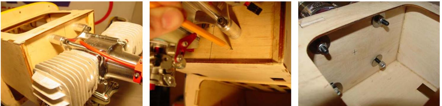
*We recommend 4/40 push rods for throttle and/or optional choke servo. Also ensure there is no metal-to-metal contact from the throttle/choke to the servos. 2/56 Ball links for 4/40 rod (not included) will prevent the aforementioned metal-to-metal contact and will bolt to nicely to your motors carburetor.*
