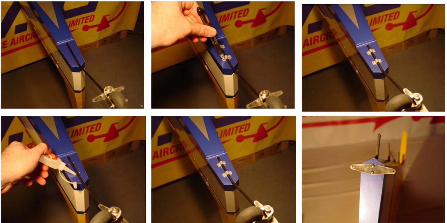
**Tip#2** Set aside your two tiller springs, we will install those later after the rudder is mounted.
